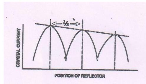
**Fig. 2** Position of Reflector vs Crystal current
